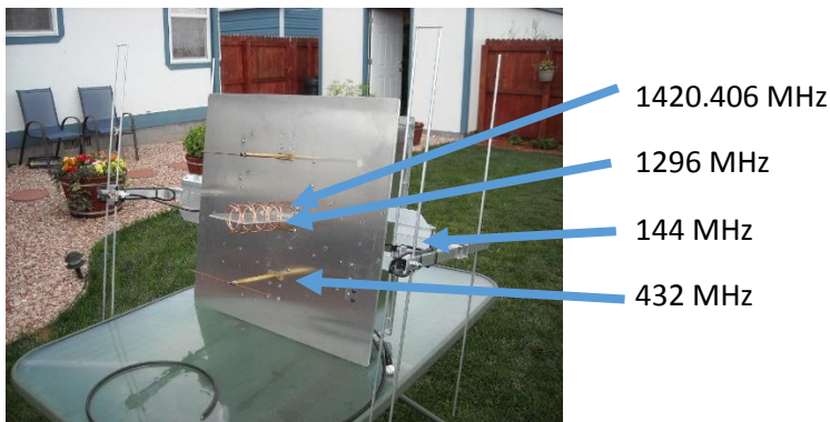
Figure 1: Multi-Band Feed
