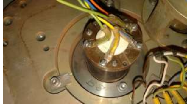
Figure 2 Dish Mount Fine 72:1 Azimuth Synchro Transmitter
