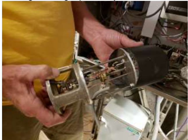
Figure 1 Dish Mount Azimuth, Limit Switch Mechanism
