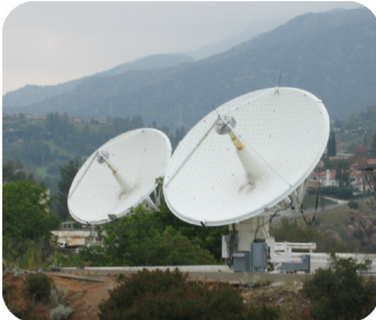
Two 6-m telescopes at JPL. Note tiny black optical telescope mounted at the lower edge of each dish.
