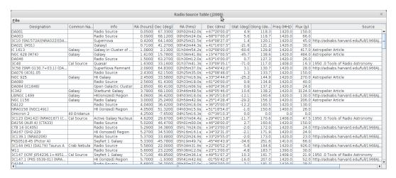
Another window contains a list of radio objects with their Right Ascension, and Declination in both decimal and H.M.S formats, Galactic Latitude and Longitude, Emission Frequency and Flux.
