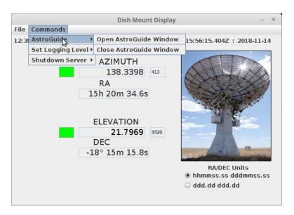
This program can be used with the System 1 controller to position the dish. The program has several different feature windows.
