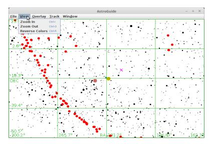
On the sky map the telescope view path can be plotted as well as most of the major objects. This make it easy to see where the dish is looking as well as make it much easier to steer the dish to and around any object of interest.
