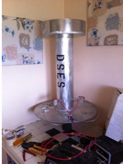
Figure 7: 21 cm Feed during assembly and Feed Installed on Pishner 18m Dish
