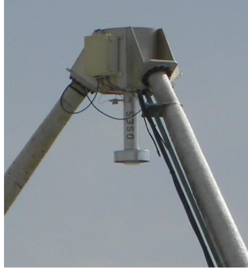
Figure 7: 21 cm Feed during assembly and Feed Installed on Pishner 18m Dish
