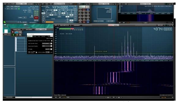
Here I synthesized the signal by modulating the 437.410 signal in steps of +/- 1500Hz with 3kHz audio modulation and received it on an SDRPlay1 software defined radio running SDR UNO.
