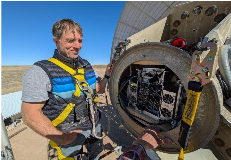
Dennis Akos from Aerospace Engineering Sciences, University of Colorado at Boulder, at the 18.3m antenna feed cavity with the new EVE 25 system inside
