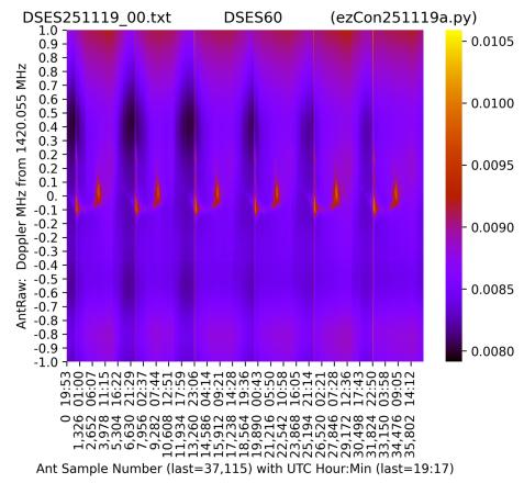
And we can plot the average value for each vertical sample line of that heat map plot (ezCon110),
