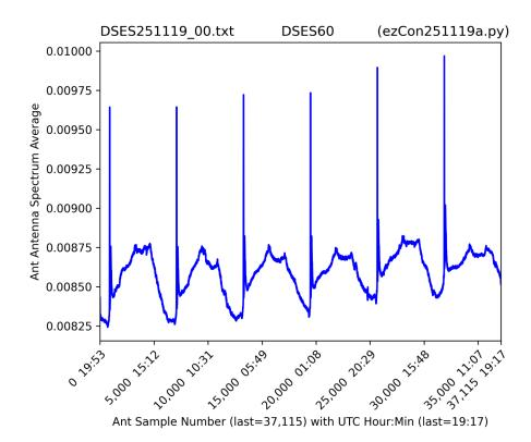
Comparing the center hydrogen frequencies to the non-hydrogen background frequencies emphasizes that Galactic hydrogen signal, to produce the AntB calculated signal (ezCon047),
